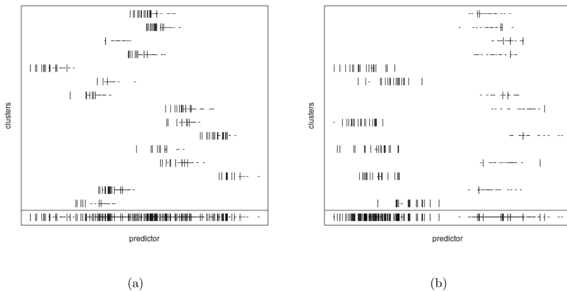
Figure 1: Two visualizations contrasting the individual and population AUCs. Each gives rug plots of fifteen clusters of data, each cluster sampled IID according to a binormal model, with the unclustered data combined at the bottom. Case observations are represented with “-” and control observations with “|”. On the left, the personalized AUC is informative and the population AUC uninformative. The reverse situation is presented on the right.
